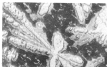
Figure 8 Annealed (700°C) alloy; Fe(35) Mn(17.5) Mo(17.5) C(30); Mo_2C + MoFe_2C + M_3C carbides. 400X
